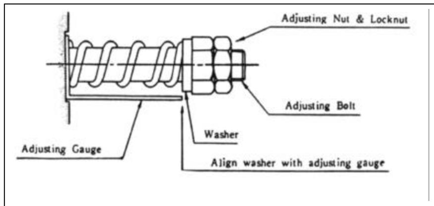
During Operation the belt may stretch causing them to slip. This will cause abrasions or cuts that can cause belts to break. Belt tension is important to ensure proper cooling tower performance and to maintain the life of the belts.
